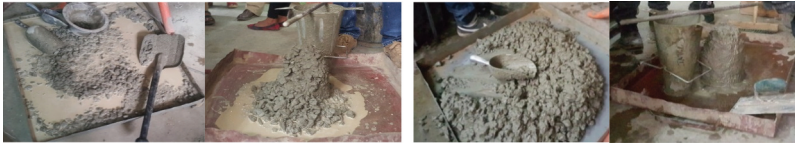
Figure 3. Highly segregated trial mix vs appropriate mix.
